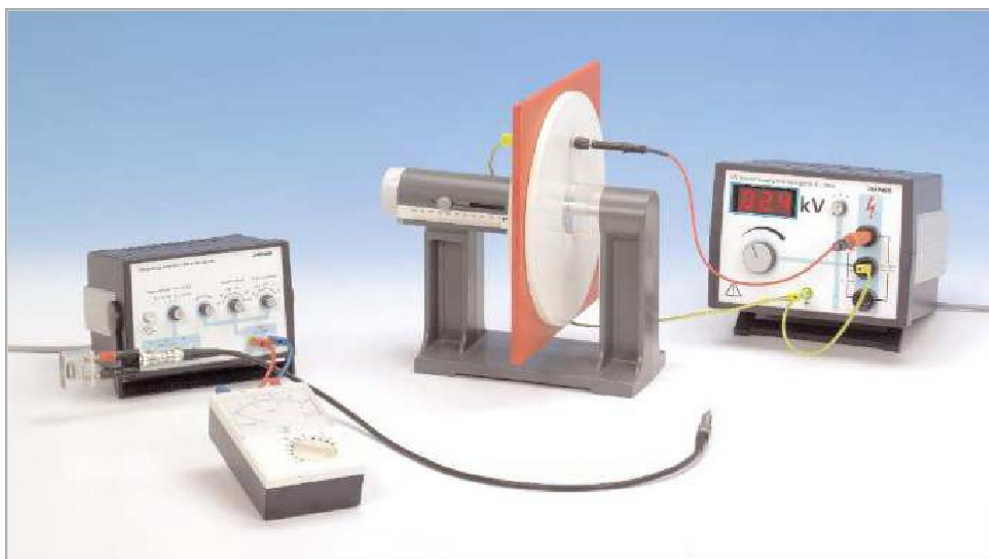
Figure 1: Measurement set-up: Dielectric constant of different materials.
