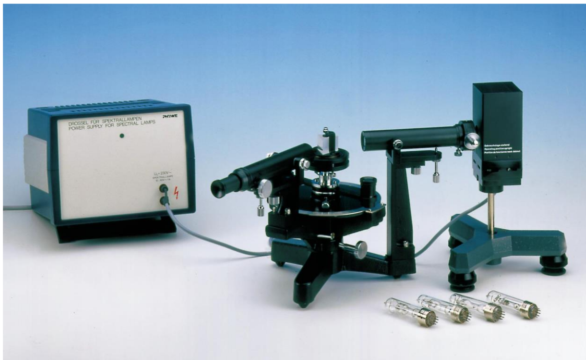
Fig.1: Experimental set up for measuring the spectra of Helium
